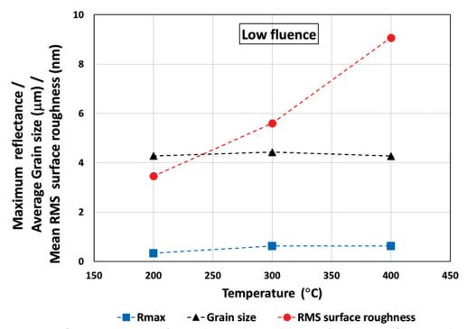
**Figure 6:** Reflectance, mean RMS surface roughness and average grain size for low neutron fluence samples irradiated at temperatures as indicated on the x-axis (dotted lines are only a guide for the eye)
