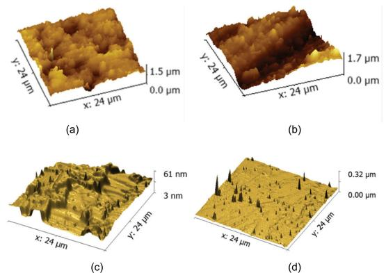
Figure 3: AFM measurements of the mean RMS surface roughness of sample 15 (a) and sample 16 (b) before polishing, and sample 15 (c) and sample 16 (d) after polishing
