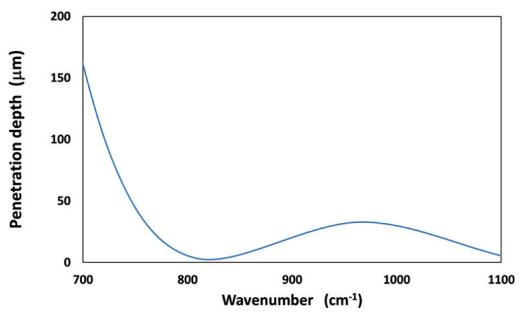
Figure 8: Penetration depth of infrared radiation in the Reststrahlen region of 3C-SiC
