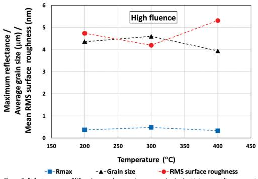
Figure 7: Reflectance, mean RMS surface roughness and average grain size for high neutron fluence samples irradiated at temperatures as indicated on the x-axis (dotted lines are only a guide for the eye)
