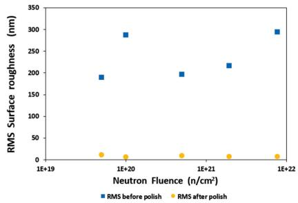
Figure 2: RMS surface roughness of all samples irradiated at 800 °C, before and after polishing
