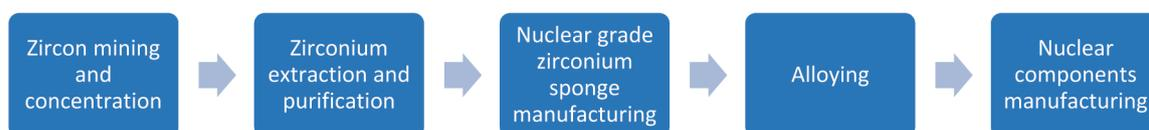
Figure 4: The main steps involved in the production of zirconium nuclear components from zircon concentrate
