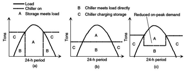
Figure 5: Operating strategies: (a) full-storage, (b) partial-storage load levelling, and (c) partial-storage demand limiting (Dincer & Rosen 2011; Selvnes et al. 2021)
