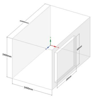
Figure 10: Dimensions of cold room
