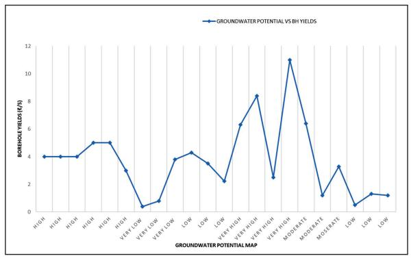
Figure 10: Correlation between produced map and actual borehole yield tests
