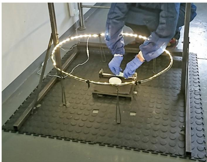
**FIGURE 1:** Stable steel frame supporting camera to photograph Nile crocodile eggs (left). An egg being placed on the matt black background and labelled with a sticker being stuck onto the Vernier (right). Note the homemade ring light to provide optimal illumination of the egg without shadows around it.
