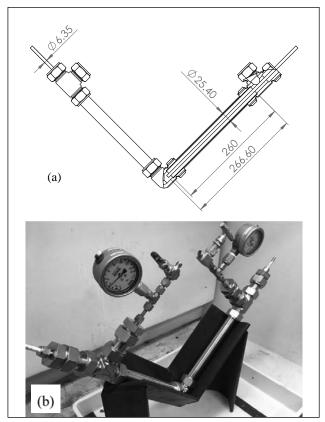
FIGURE 5: (a) Mechanical design sketch, and (b) a photograph of the fluorine cell
