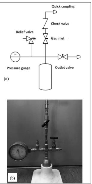
FIGURE 4: Anhydrous HF transfer vessel: (a) P&ID; (b) photograph of the vessel in a 3D-printed stand
