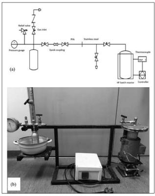
FIGURE 3: HF batch reactor experimental setup: (a) P&ID; (b) photograph
