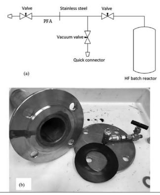
FIGURE 2: HF batch reactor: (a) P&ID of the setup; (b) a photograph of the reactor
