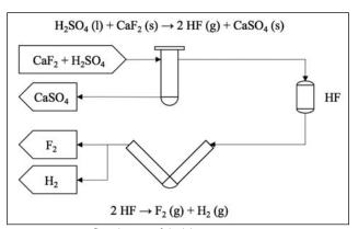
FIGURE 1: Process flow diagram of the laboratory system
