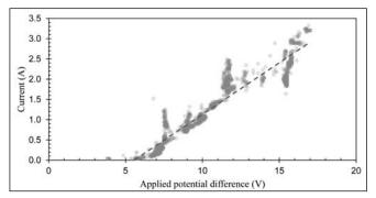
FIGURE 7: Fluorine voltametric data, experiment F2
