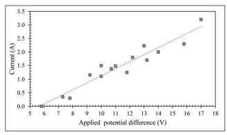
FIGURE 6: Fluorine cell voltametric curve, experiment F1
