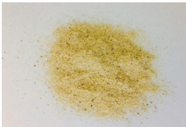
Figure 1: Picture of a treated and milled sisal fibre (Phiri, 2012)
